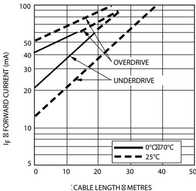
Figure 4: Guaranteed System Performance with Improved Cable (HFBR-15X1Z/25X1Z)
