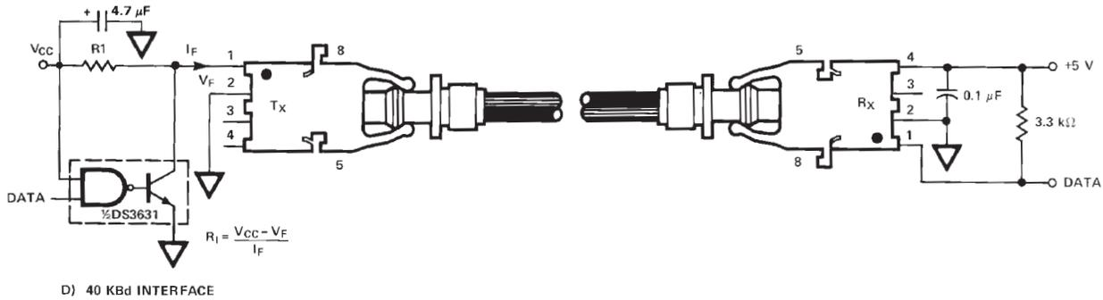
Figure 21: Guaranteed System Performance with Standard Cable
