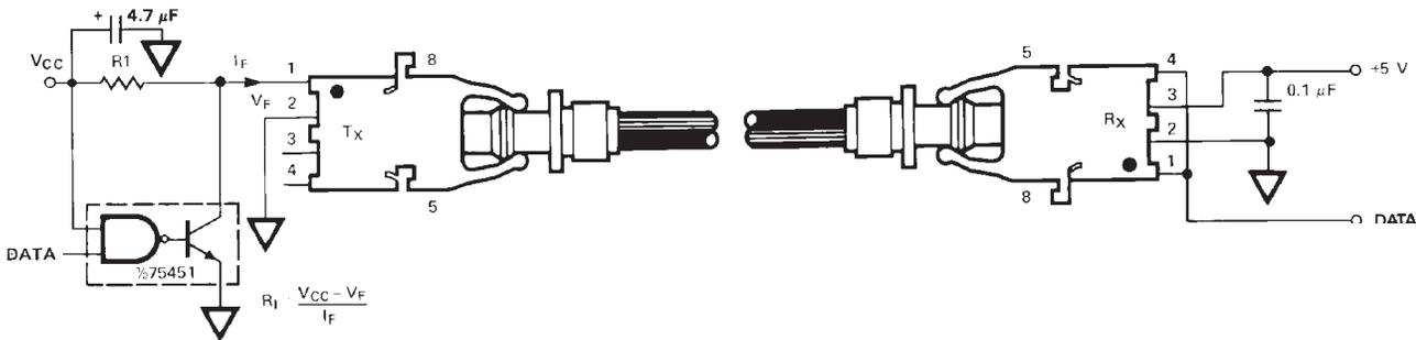
Figure 3: Guaranteed System Performance with Standard Cable (HFBR-15X1Z/25X1Z)
